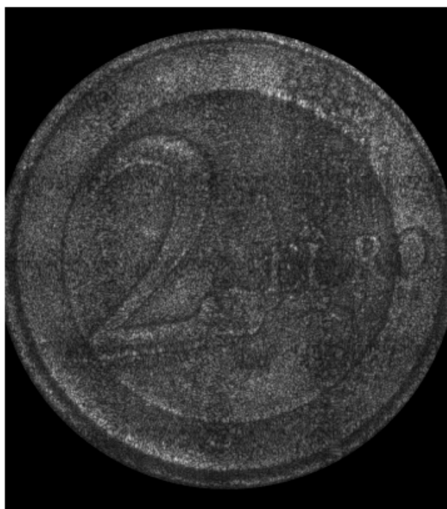
Figure 29 : Hologram reconstructed by convolution
