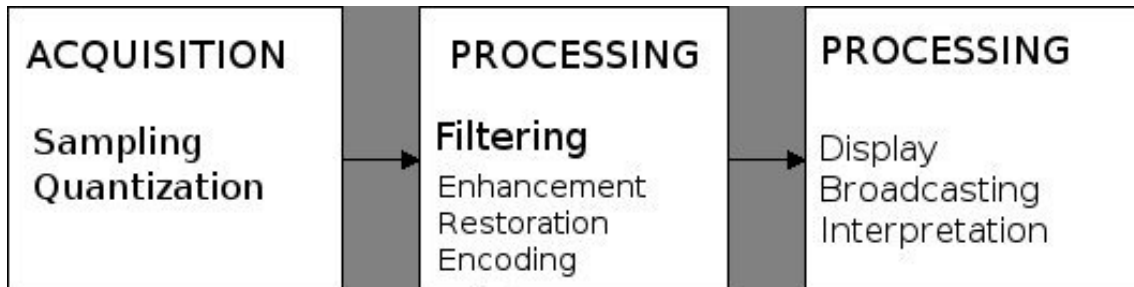
Figure 1: General diagram of the image processing chain.
